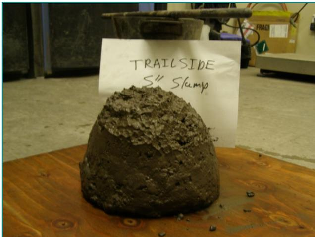
Trailside Sample Slump Test
