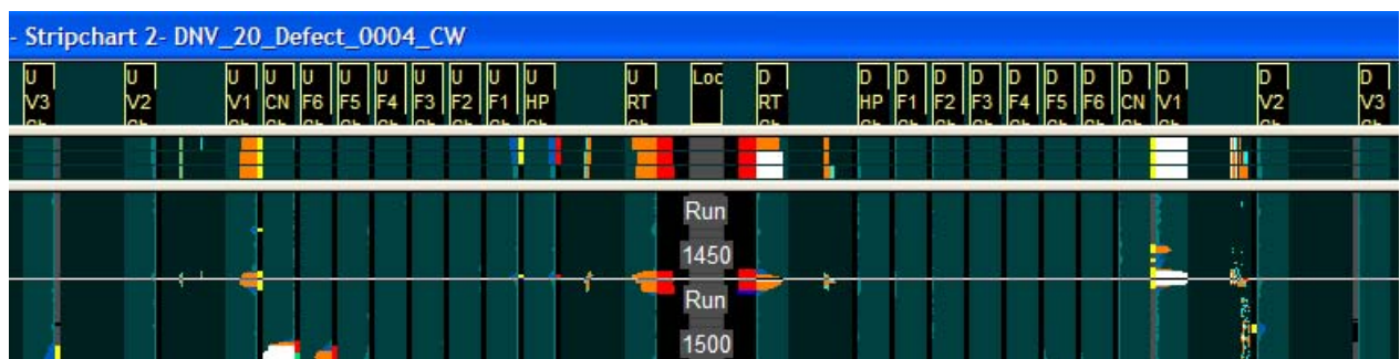
Figure 14: Root indication in Defect 4-7 at position 1464 mm. Macro indicates a defect height of 3.1 mm, height has been interpreted to between 2.0 and 2.5 mm from AUT scan. US-side to right on macro.
