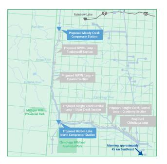
The proposed 15 megawatt Hidden Lake North Compressor Station would be located at the west end of the proposed Tanghe Creek Lateral Loop (Sloat Creek Section) located at SW 32-96-11-W6M, approximately 140 km northwest of Manning, Alberta.
