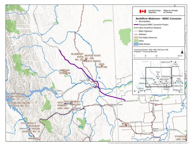
On 18 November 2021, NorthRiver filed the Application (<u>C16186</u>) for the NEBC Connector Project pursuant to sections 182 and 183 of the CER Act. The Project consists of two parallel pipelines that are each approximately 215 km in length. The pipeline components for the Project require a total cumulative length of approximately 215 km of RoW, approximately 20 km of which will be new non-parallel RoW, as well as associated temporary workspace.
