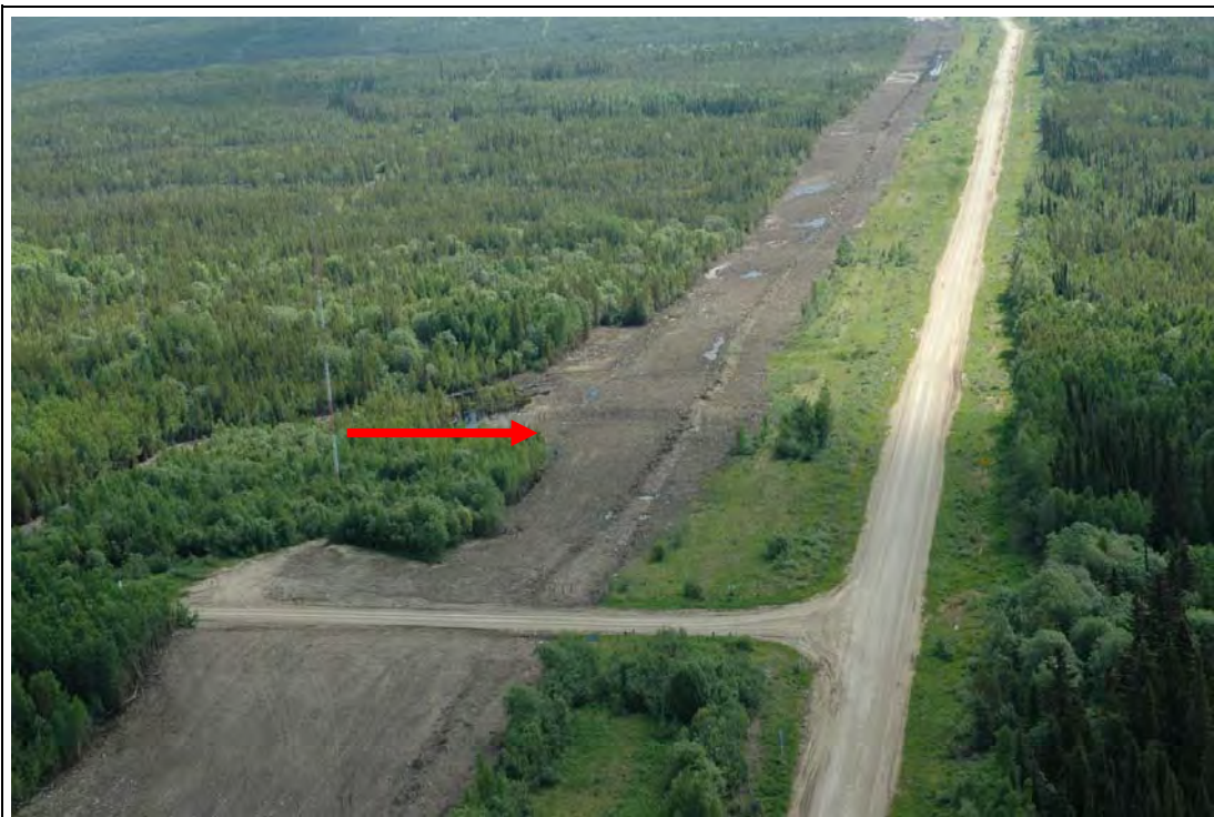
Plate 26 Example of multiple existing linear disturbances that facilitate access (roads, pipeline right-of-way). Access management (earth berm) on the new paralleling pipeline right-of-way is unlikely to be effective. Photo source: CH2M HILL.
