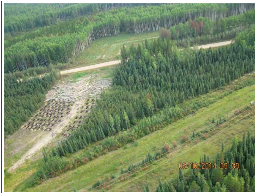
Plate 14 Example of a combination of access management measures: rollback (upland/transitional area) and mounding (lowland area). The volume of woody debris at this location was increased to comply with regulatory request. The coverage in this location, while effective for access management, is excessive for facilitating vegetation establishment. Photo source: NGTL.
