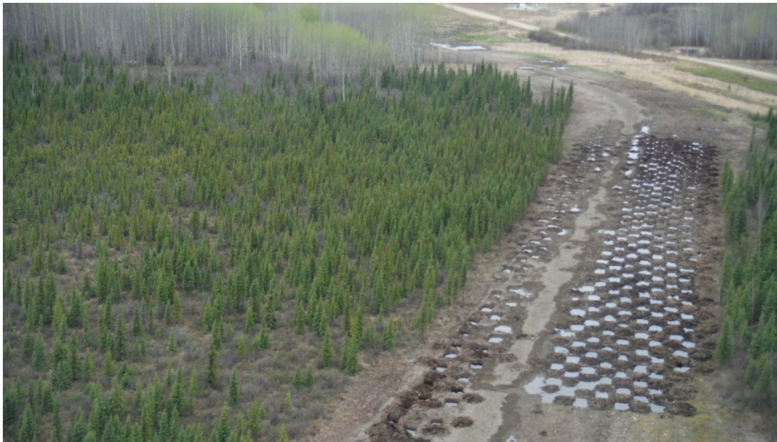
Plate 5: Aerial view of mounding in lowland on a non-parallel portion of the ROW. Photo source: NGTL.
