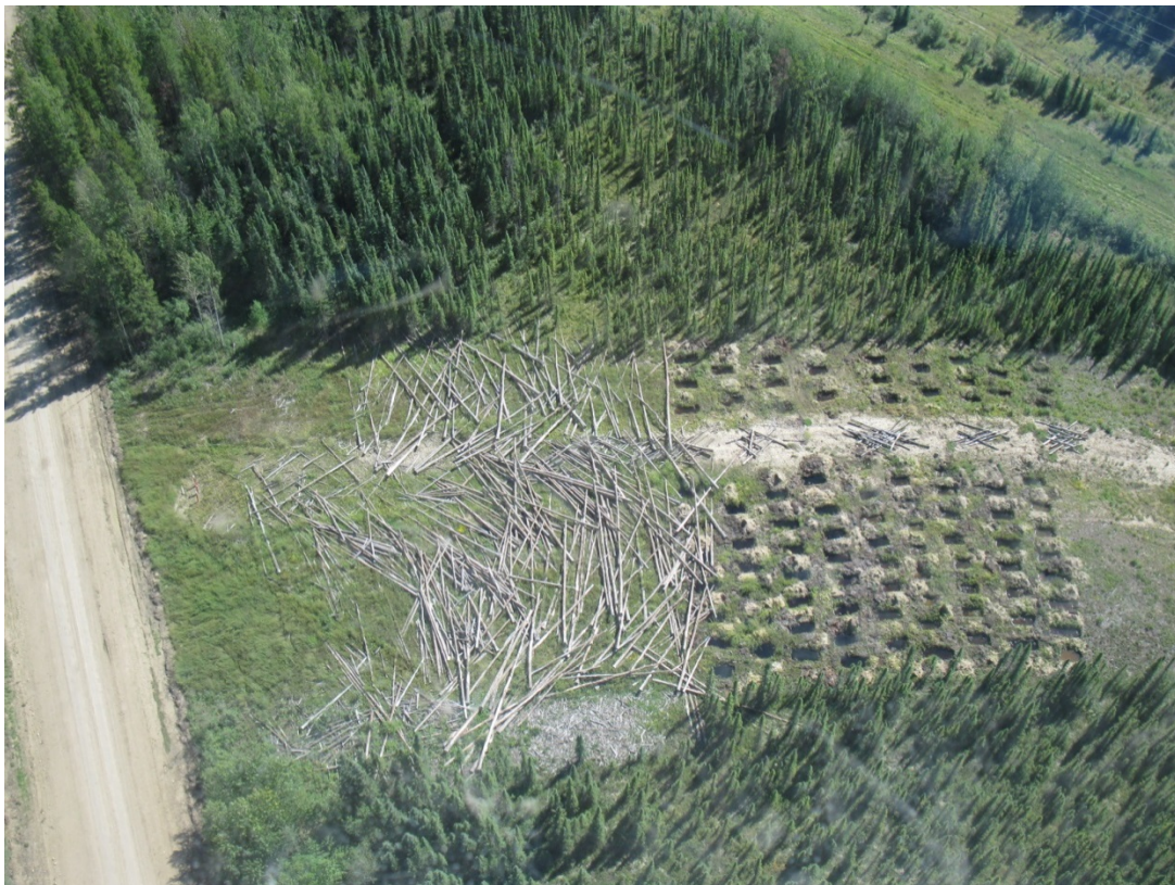
Plate 6: Aerial view of combination rollback and mounding as access management on a non-parallel portion of the ROW. Photo source: NGTL.
