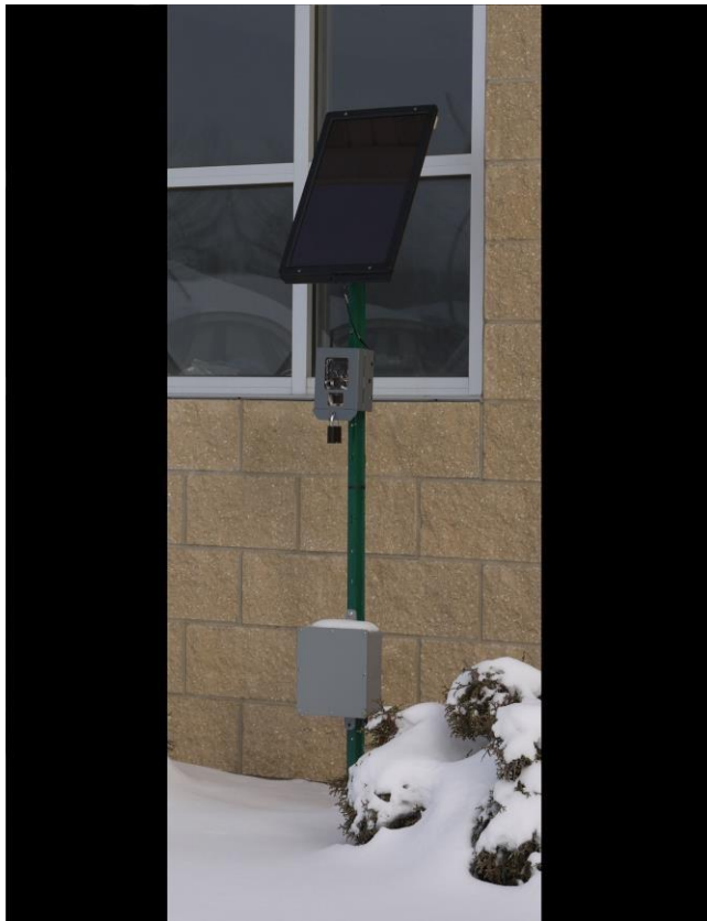
Photo 1: Example Camera and Solar Power Panel Pack Mounted on a T-post (© Reconyx)
