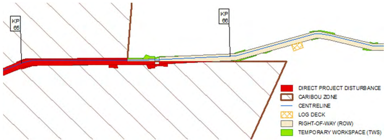
Figure 2 Example of Direct Project Disturbance
