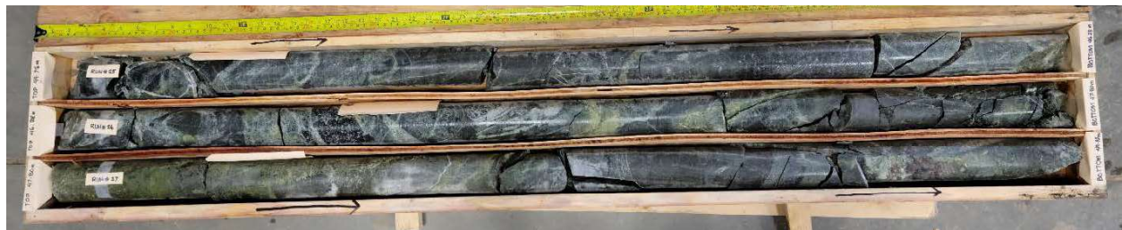
PHOTO 15 TEL-JL-BH14 RUN 25-27 (44.72 to 49.30 m)
