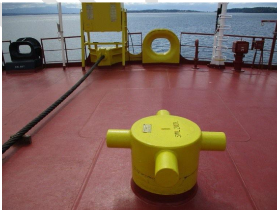
Figure 7: Examples of vessel's towing strong points that are suitable for escort tug line securing.
