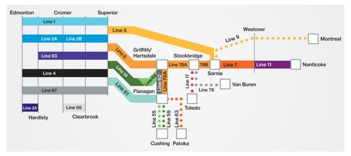
Note: Canadian Mainline and Lakehead system pipelines are denoted in solid colours. Pipelines denoted with a dotted line are not part of the Enbridge Mainline system.
