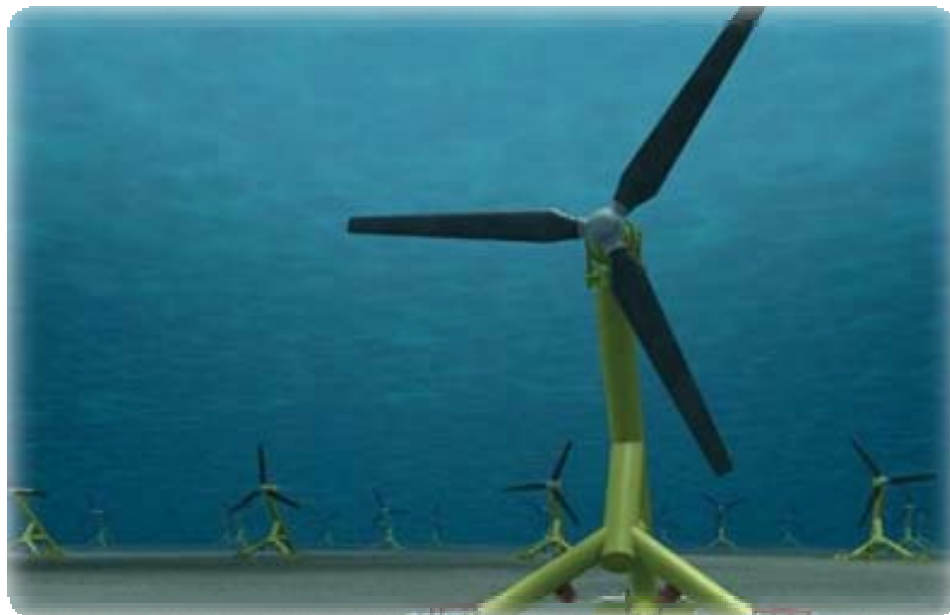
Figure 38: Typical bottom mounted axial tidal stream turbine
