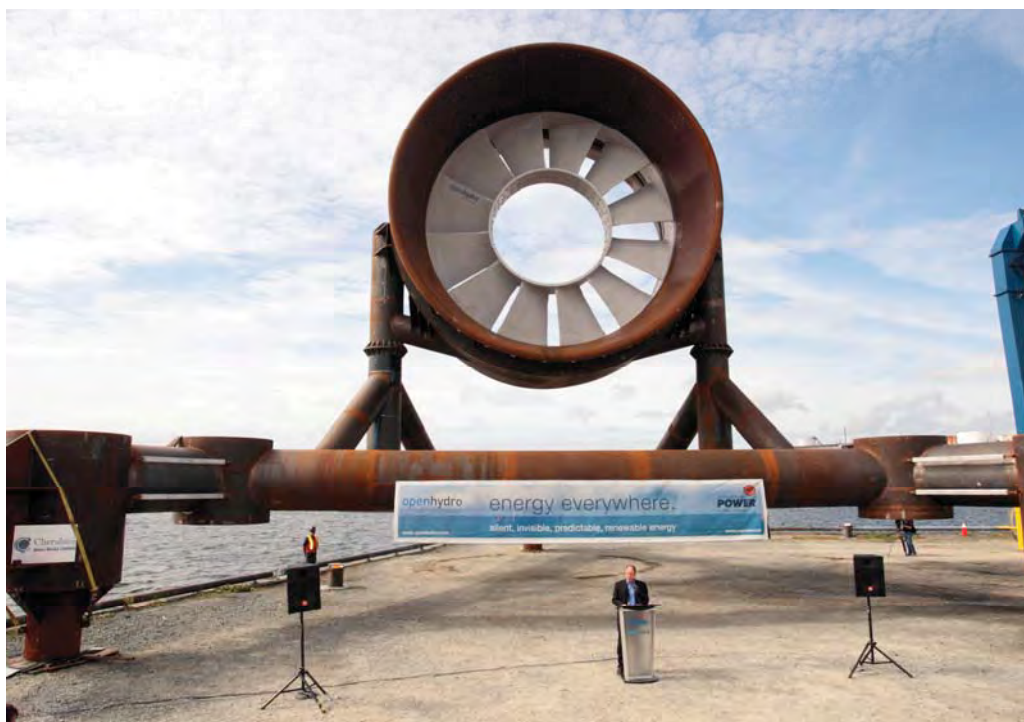
Figure 37: In-stream tidal turbine used in Nova Scotia
